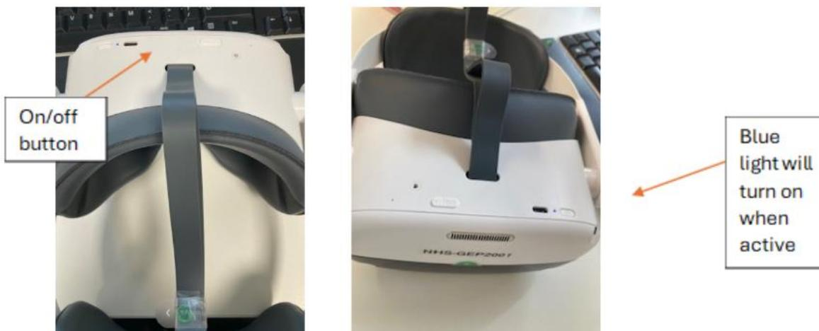
Once powered up, the headset should open on the home screen with a view of the earth, a tree, a sofa and bookcase. If the control panel menu is not visible, it can be displayed by using the bottom circle button on the right side of the headset. The larger button above this is the selection button – pressing this enables you to make a selection, like the left click button on a computer mouse.
